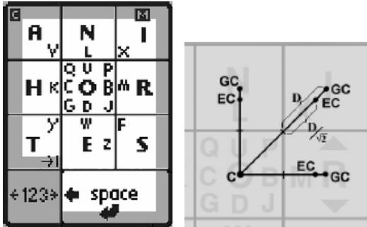
**Figure 6. (a) Effective area of the keyboard for typing letters + space, (b) Finding the effective center (EC).**
